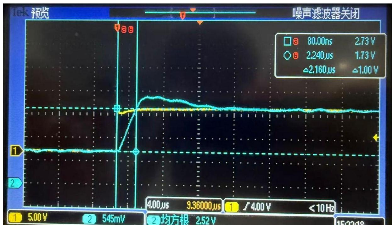
Fig.3 CH1 is primary magnetic field, and CH2 is output voltage; FFE-002F16LV5JR-020K series show output response time of 2.16 μs (~2 μs)
